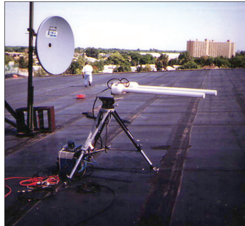
Figure 2.114 A common sight above large events. The blimp usually has an omnidirectional antenna to transmit its camera signal back to the ground. The receive site on the ground often has a steerable antenna, this one under manual control.
