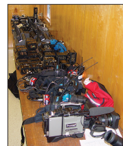
Figure 2.106 Here is a small part of the RF equipment used at the Indianapolis 500. At the bottom of the photo is one of the many wireless cameras that wandered the pit area. The box comprising the rear third of the camera, with the whip antenna, controlled camera operating parameters via telemetry received by the antenna. Behind the camera are a number of "talent packages" that included a wireless mic and IFB. Un-tethered, free-ranging cameras need power, so as we walk down the table past the mics we come to a pile of batteries that clip onto the back of the camera. At the far end are a slew of handheld radios in their chargers.
