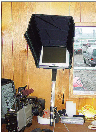
Figure 2.113 Flat-panel display that served as program monitor for the roving talent at the Indy 500 race. This display is part of a "roving" kit shown in Figures 2.101 and 2.103.
