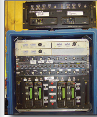
Figure 2.109 This BST flight case has IFB interfaces with the compound's IFB/intercom (top), which emanates from the main production truck. Program audio is also fed in and processed to the talent's preferences and handed off to the radios at the bottom.
