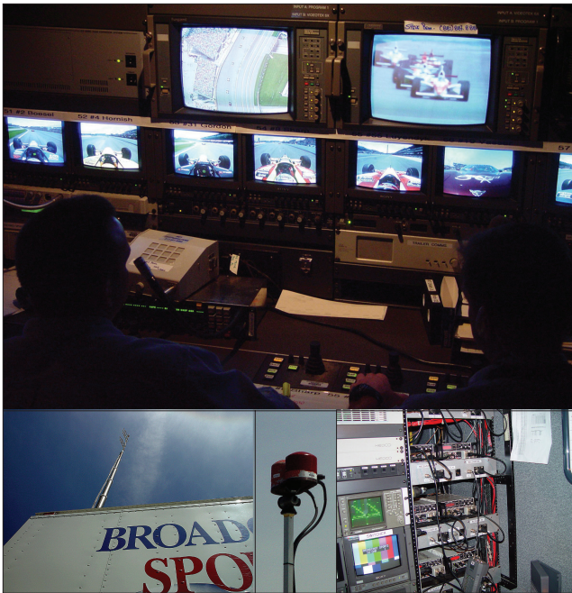
Figure 2.108 In-car cameras provided by BST. BST brings its own trailer, housing camera control and RF electronics, to the venue. The operators shown at top can pan and tilt the camera, and control camera attributes such as iris and black level, as well as "paint" the camera. These operators can also control what frequency each car's transmitter is using, and advance the clear screen in front of the camera lens that is continuously peppered with track debris. Each car, up to eight, transmits up to a helicopter that hovers overhead and relays the signal down to redundant receive antennas on top of the trailer (bottom center). The raised mast, also on top of the trailer (bottom left), is for telemetry between the trailer and the cars.
